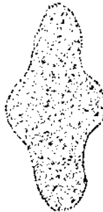
Figure 33. Heavy Center Pattern
