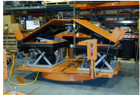
2 Rack positions with lift & tilts
