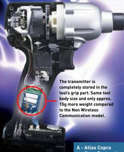
The transmitter is completely stored in the tool's grip part. Same tool body size and only approx. 15g more weight compared to the Non Wireless Communication model.
