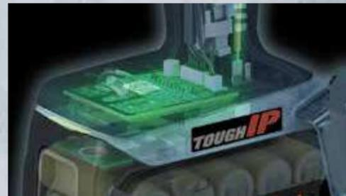
The circuit detects battery voltage, controls the proper current and delivers the correct voltage flow to the tool for best performance
