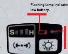
Flashing lamp indicates low battery.
