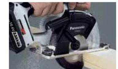
3 Eject dust to the rear of the machine
