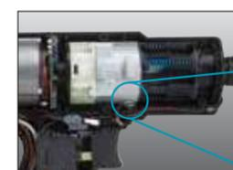
Sensing the clutch plate movement, the Photo Interrupter Sensor increases clutch life and tool accuracy not relying on mechanical contacts that wear.
