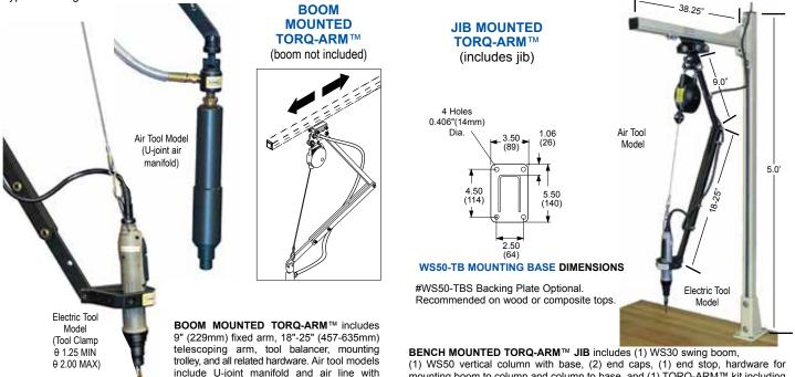
(1) WS50 vertical column with base, (2) end caps, (1) end stop, hardware for mounting boom to column and column to base, and (1) TORQ-ARM™ kit including 9" (229mm) fixed arm, 18"-25" (457-635mm) telescoping arm, tool balancer, mounting trolley, and all related hardware. Air tool models include U-joint manifold and air line with fittings. Electric tool models include tool clamp.
