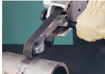
Model 11475 is ideal for grinding circumferential welds.
