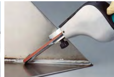
Grind welds using belts as narrow as 1/8" wide.
