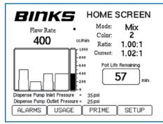
Home Screen provides real time data and displays vital information such as Flow Rate, Pot Life, Current Mix Ratio, and Current Color. The Home Screen is always accessible by pressing the lower left button on the pendant. This dedicated button simplifies user navigation.
