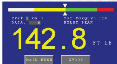
Example shows testing a 250 ft.lb. wrench at 60% of full scale. Yellow indicates low reading.
