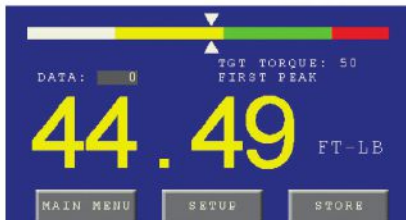
Example shows testing a 250 ft.lb. wrench at 20% of full scale. Yellow indicates low reading.
