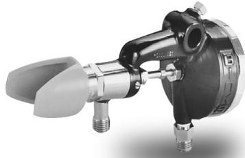
For spraying protective coatings such as lacquers, enamels, water-based emulsions, mold release agents, and sound deadeners. Spray gun equipped with tip guard, stainless steel fluid passages, and forged aluminum spray gun body. Actuating air pressure is 40-60 PSI. The material body may be installed in any of four positions to facilitate fluid hose connection. Spray nozzle not included, order separately. Mounting hole is 1/2" diameter, furnished with set screw.
