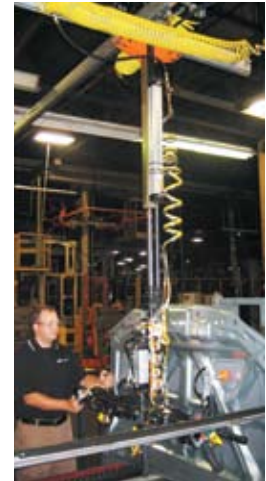
Torque tube with integrated vacuum handling device
