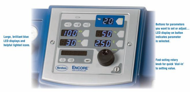
Powerful Performance Package of Encore<sup>™</sup> Control System: Digital Closed-Loop Fl
